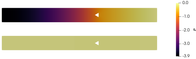
FIGURE 13: REAL (TOP) AND IMAGINARY (BOTTOM) COMPONENTS OF THE ACOUSTIC PRESSURE EIGENFUNCTIONS OF THE 1ST MODE FOR THE FLAME AT t = 310 AND AMPLITUDE \epsilon_0 . THE EIGENFUNCTION IS NORMALIZED SUCH THAT \int p^2 dx = 1 .
